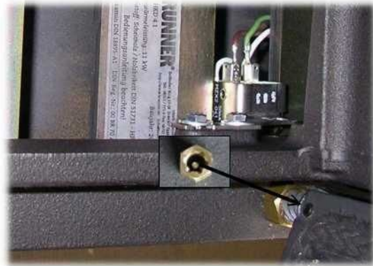
Illustr. 4: Door switch installed
