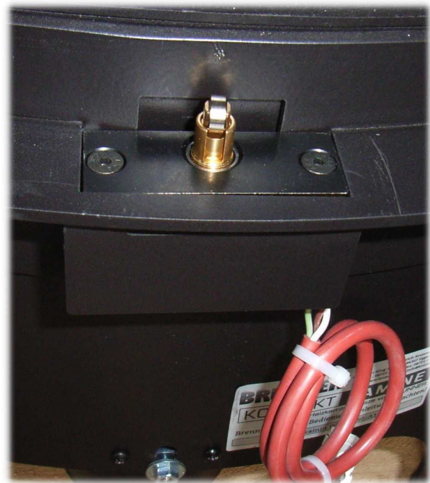
Illustr. 17: Door switch installed
