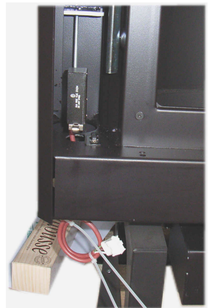
Illustr. 23: Door switch installed
