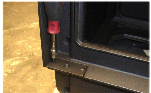
Illustr. 10: Mounting plate removal
