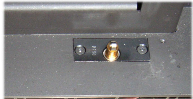
Illustr. 30: Door switch installed
